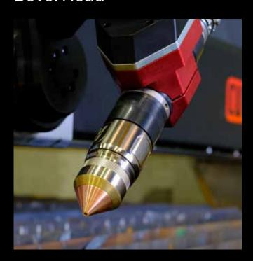
Utilising the Hypertherm XPR plasma system, cut angles of up to  $\pm 50^{\circ}$  can be achieved with unlimited winding.
