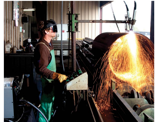
Pipe cutting and beveling
